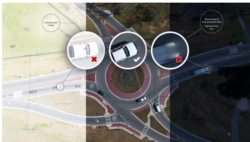
Figure: Three situations – nok: too bright (left), ok: ideal (center), nok: dark, blurred due to long exposure time (right).
