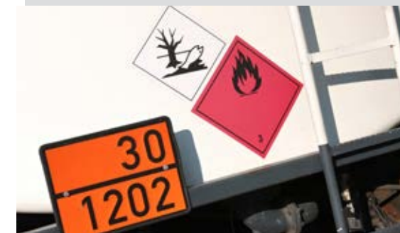
ADR = Dangerous goods recognition Automatic registration of dangerous goods transports and their cargo types, reads written and empty signs.
