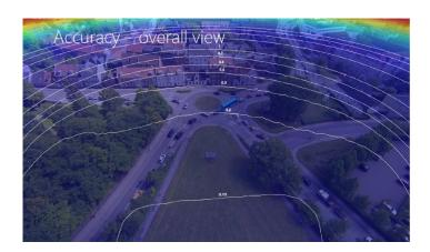
Accuracy of localization with a view from a drone. Contours within the image represent the possible object localization accuracy at the given part of the image (up to 15 cm!).
