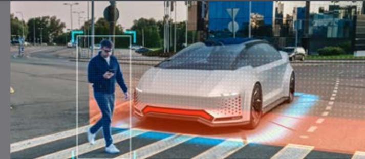
Autonomous driving: Detection of a pedestrian triggers automatic vehicle braking.
