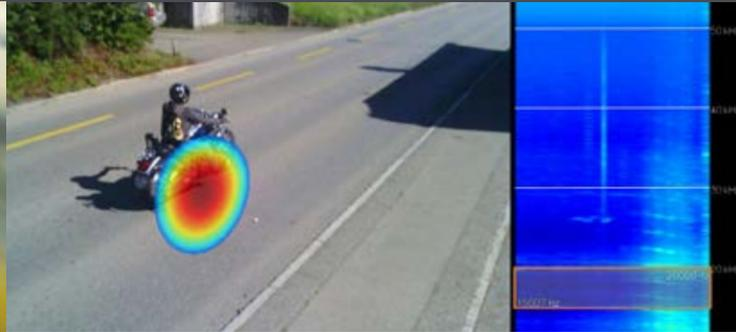
Detection and Determination of Noise at the Source.
