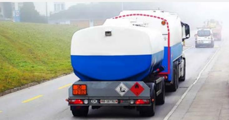
Hazardous goods transport in Switzerland with cargo labeling using an orange sign.
